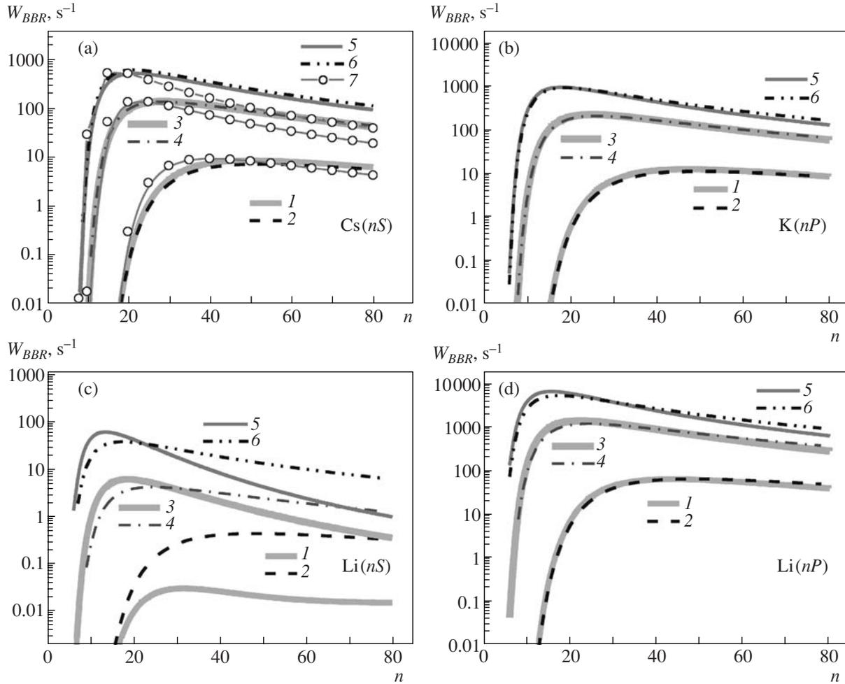
**Fig. 2.** Dependences of the direct blackbody photoionization rate  $W_{BBR}$  on the principal quantum number  $n$  calculated numerically (curves 1, 3, and 5) and analytically (curves 2, 4, and 6) at  $T = 77, 300,$  and  $600$  K for Rydberg atoms: (a)  $nS$  cesium, (b)  $nP$  potassium, (c)  $nS$  lithium, and (d)  $nP$  lithium. Curve 7 in (a) is the calculation by the analytical formula from [9] for these temperatures.
