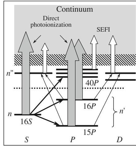
**Fig. 1.** Schematic diagram of ionization of the lithium atom in the  $16S$  Rydberg state by blackbody radiation (SEFI is the selective electric-field ionization; high-lying Rydberg states are in the hatched region).
