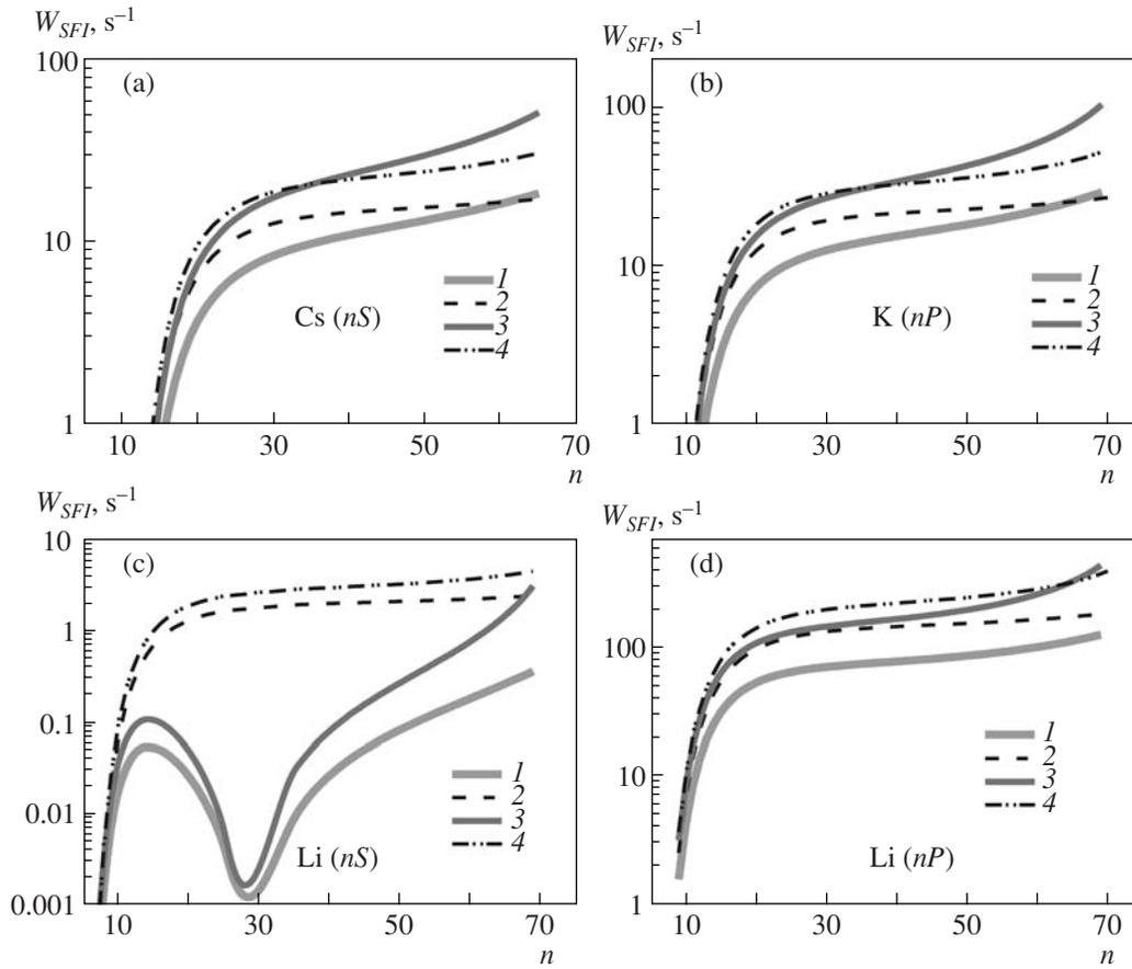
**Fig. 3.** Dependences of the photoionization rate  $W_{SFI}$  by electric pulses on the principal quantum number  $n$  calculated numerically (curves 1 and 3) and analytically (curves 2 and 4) at  $T = 300$  K and electric field amplitudes of 5 and 10 V/cm for Rydberg atoms: (a)  $nS$  cesium, (b)  $nP$  potassium, (c)  $nS$  lithium, and (d)  $nP$  lithium. Ionization occurs as a result of population of high-lying Rydberg states induced by the blackbody radiation.
